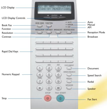
The user-friendly fax control panel provides users with quick access to features.
